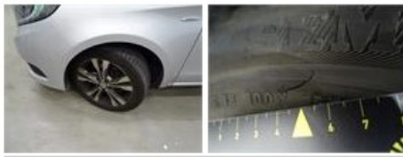
Alloy rim R R polished, Damaged, E - Replace 182,40
