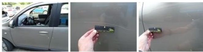
Door frame F L, Bump(s) and scratch(es), It - Spot repair 115,56
