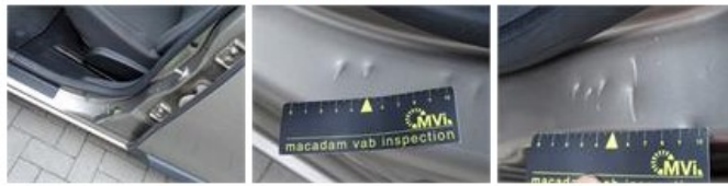
Bonnet, Bump(s) and scratch(es), LI - Repair and paint (complete) 232,06
