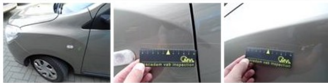
Reflector, Damaged, E - Replace 15,00
