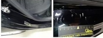
Rocker panel inner R R, Bump(s) and scratch(es), LI - Repair and paint (complete)
