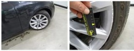
Alloy rim R R, Scratch(es), LI - Repair and paint (complete) 95,00
