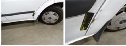
Wing F L, Scratch(es), It - Spot repair
