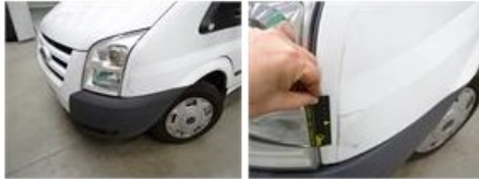
Wing F L, Scratch(es), It - Spot repair
