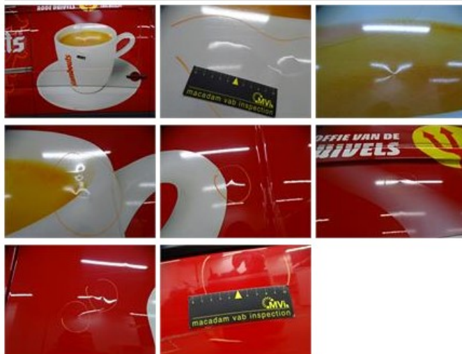
Door R R, Bump(s) and scratch(es), LI - Repair and paint (complete) 238,76
