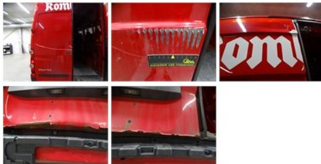
Spare wheel compartment lining R R, Bump(s), Smart repair 110,64
