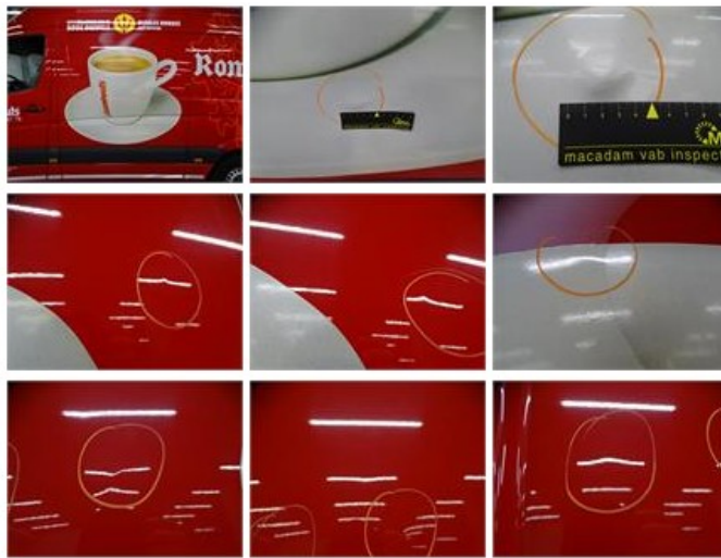
Trunk door R L, Damaged, Le - Replace and paint 446,00
