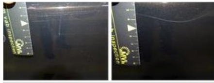
Rocker panel inner R L, Bump(s) and scratch(es), LI - Repair and paint (complete)
