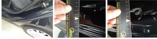
Rocker panel inner R L, Bump(s) and scratch(es), LI - Repair and paint (complete)
