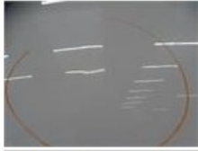
Door R R, Bump(s) and scratch(es), LI - Repair and paint (complete) 318,35
