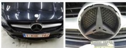
Bumper grille F L, Missing, E - Replace 32,40
