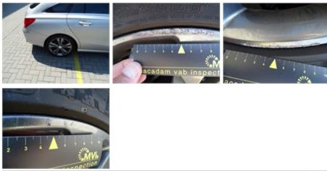
Alloy rim F R, Damaged, E - Replace 235,20
