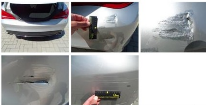
Front bumper, Tear, Smart repair 110,64
