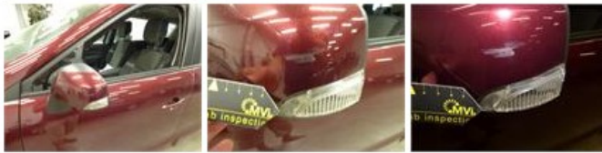
Rearview mirror glass L, Damaged, E - Replace 18,00
