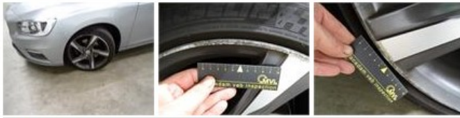
Alloy rim F R polished, Scratch(es), LI - Repair and paint (complete) 95,00
