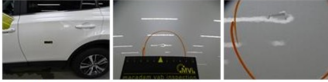
Door R L, Bump(s) and scratch(es), LI - Repair and paint (complete) 318,35
