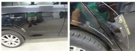
Wing F R, Bump(s) and scratch(es), Le - Replace and paint 530,02
