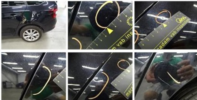
Door R R, Bump(s) and scratch(es), LI - Repair and paint (complete) 318,35
