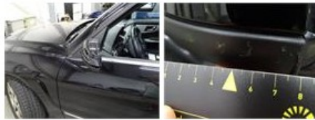
Sill outer L, Scratch(es), It - Spot repair 115,56
