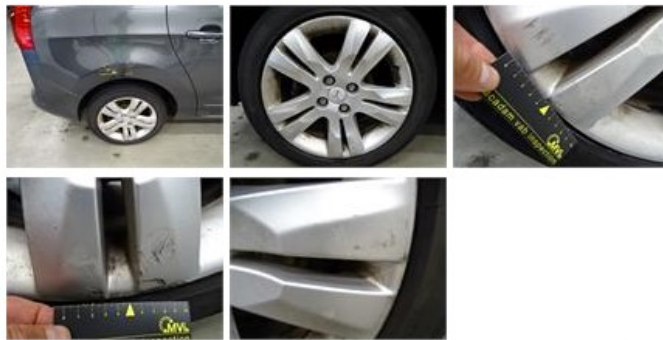
Protection plate M, Tear, E - Replace 74,00
