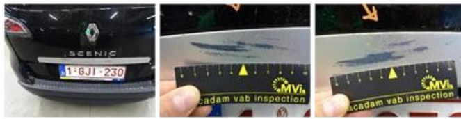
Protection plate M, Tear, E - Replace
