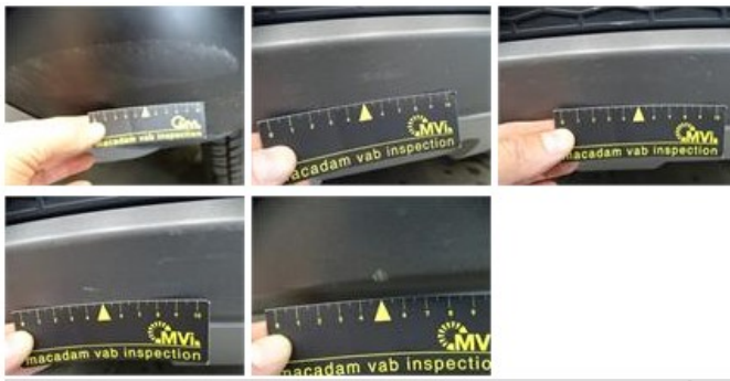
Door R R, Bump(s) and scratch(es), LI - Repair and paint (complete) 0,00
