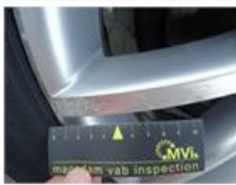
Alloy rim R R, Rust, LI - Repair and paint (complete)
