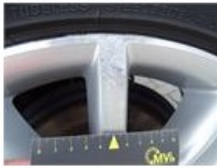
Alloy rim R L, Rust, LI - Repair and paint (complete)
