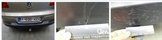
Bumper grille, Damaged, E - Replace
