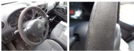
Wheel cover F L, Missing, E - Replace
