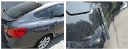
Door panel R R, Damaged, Smart repair 110,64
