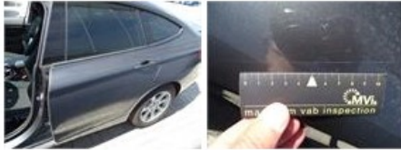
Door R L, Scratch(es), LI - Repair and paint (complete) 382,02
