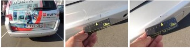
Bodywork, Not original part, P - Check
