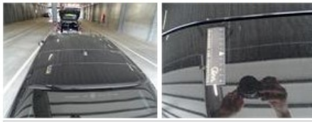
Roof, Scratch(es), LI - Repair and paint (complete) 481,50
