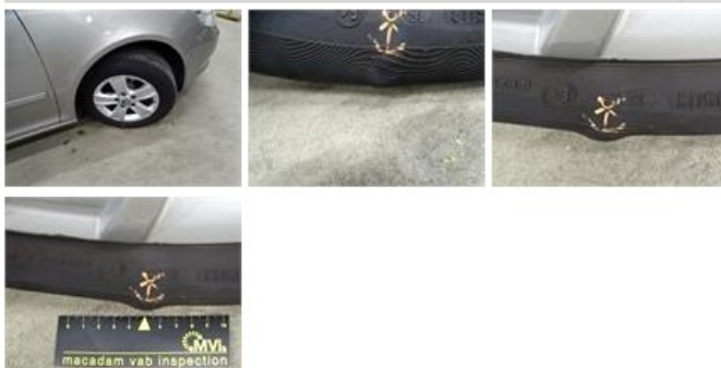
Sill outer L, Bump(s) and scratch(es), LI - Repair and paint (complete) 310,50
