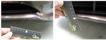
Door R L, Dent(s) and scratch(es), LI - Repair and paint (complete) 414,35
