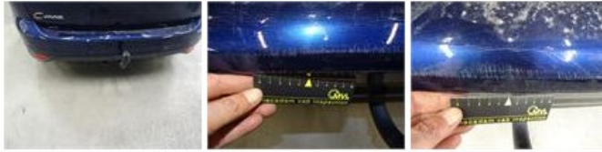
Bumper grille, Broken, E - Replace 54,00
