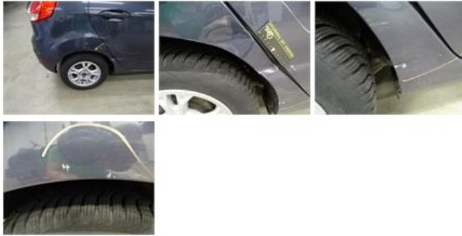
Wing R R, Dent(s) and scratch(es), Le - Replace and paint 1033,21
