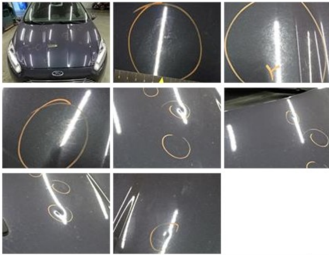
Wing R R, Dent(s) and scratch(es), Le - Replace and paint 1033,21
