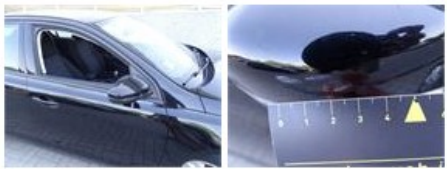
Sill outer R, Dent(s) and scratch(es), LI - Repair and paint (complete) 502,50
