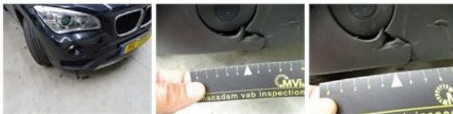
Front bumper, Dent(s) and scratch(es), Smart repair 110,64
