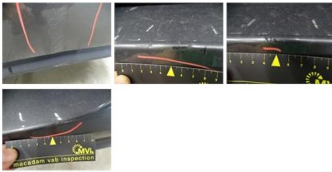
Door F L, Dent(s) and scratch(es), LI - Repair and paint (complete) 382,02
