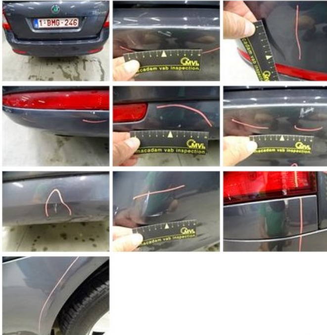
Wing F R, Scratch(es), LI - Repair and paint (complete) 220,18
