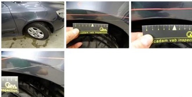
Wing R L, Scratch(es), LI - Repair and paint (complete) 308,20
