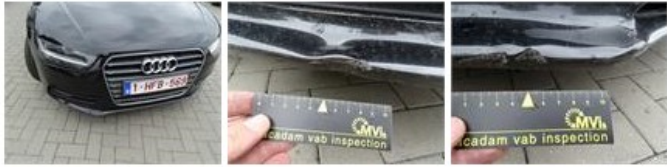
Front bumper, Dent(s) and scratch(es), Le - Replace and paint 735,00
