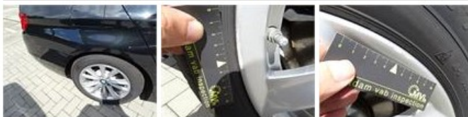
Door F L, Scratch(es), It - Spot repair 115,56
