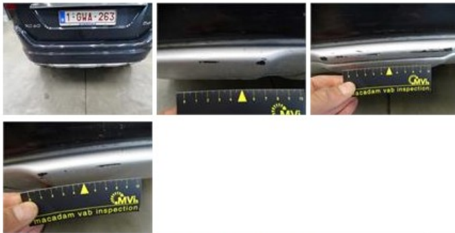
Wing R R, Scratch(es), LI - Repair and paint (complete) 369,84
