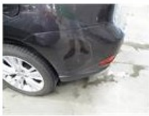
Bumper R, Crack, Le - Replace and paint
