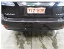
Bumper R, Crack, Le - Replace and paint
