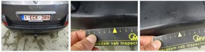
Door R R, Dent(s) and scratch(es), LI - Repair and paint (complete) 254,68
