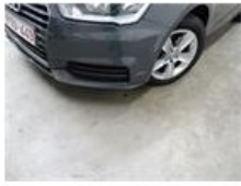
Front bumper, Dent(s) and scratch(es), LI - Repair and paint (complete) 169,44
