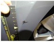
Front bumper, Dent(s) and scratch(es), LI - Repair and paint (complete) 169,44
