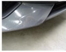
Front bumper, Dent(s) and scratch(es), LI - Repair and paint (complete) 169,44
