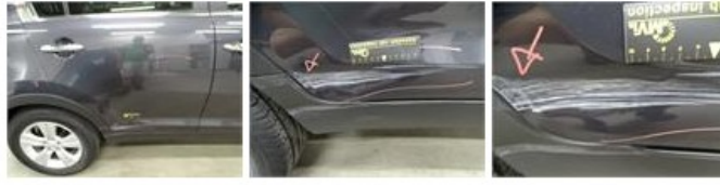
Door R R, Dent(s) and scratch(es), LI - Repair and paint (complete) 318,35
