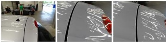
Wing R R, Hail damage, LI - Repair and paint (complete) 246,56
