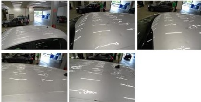
Wing R L, Hail damage, LI - Repair and paint (complete) 246,56
