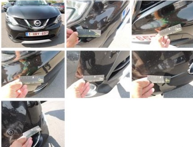
Bonnet, Stone chip(s), LI - Repair and paint (complete) 290,08
