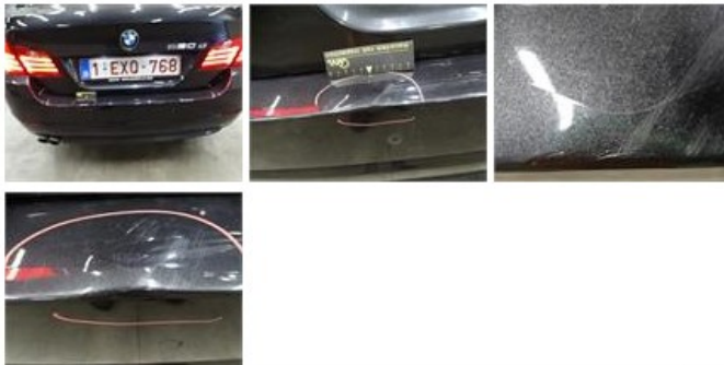
Tailgate, Bad repair, Acceptable
