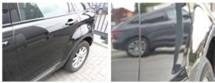
Door R R, Dent(s) and scratch(es), LI - Repair and paint (complete) 382,02
