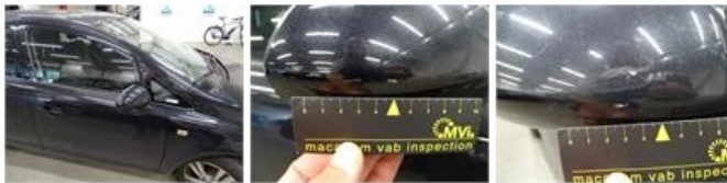
Door R R, Scratch(es), LI - Repair and paint (complete) 254,68
