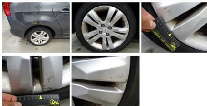
Protection plate M, Tear, E - Replace 74,00
