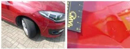
Wheel cover F R, Broken, E - Replace 0,00
