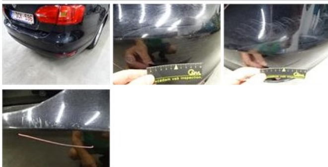
Door R R, Dent(s) and scratch(es), LI - Repair and paint (complete) 318,35
