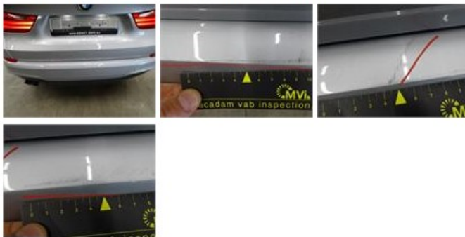
Rearview mirror housing L, Scratch(es), Acceptable 0,00
