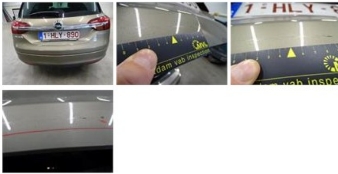
Tailgate, Scratch(es), LI - Repair and paint (complete) 301,68
