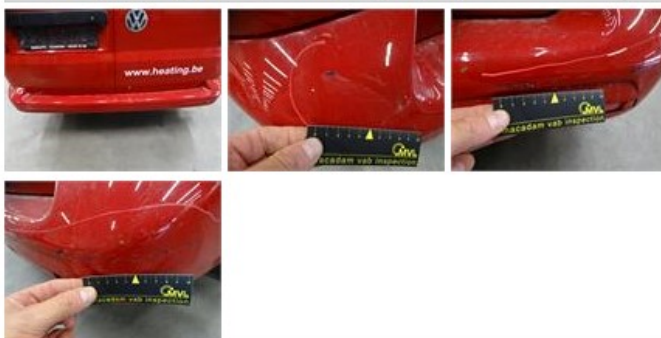
Wing R R, Scratch(es), LI - Repair and paint (complete) 231,15
